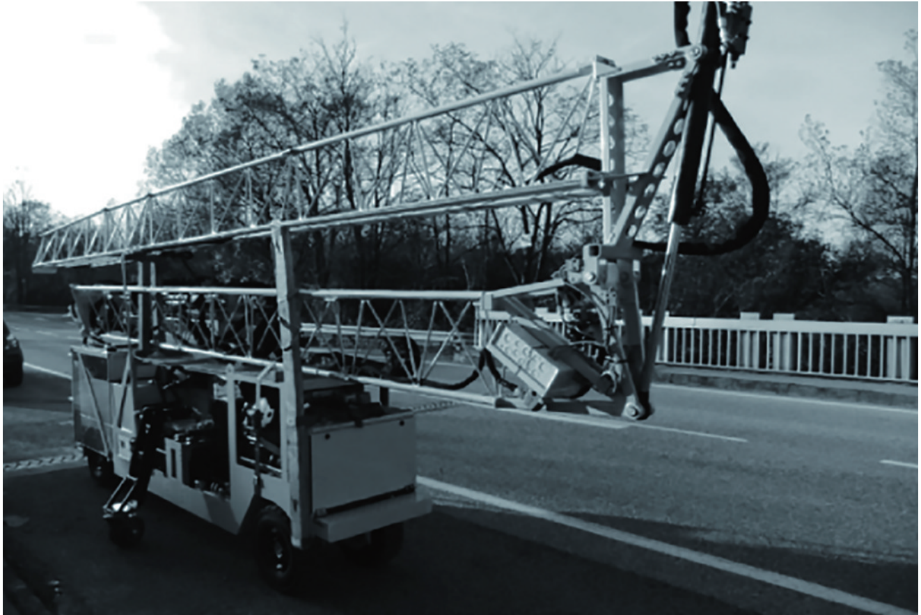
Fig. 7 Bridge beam-bottom inspection robot
