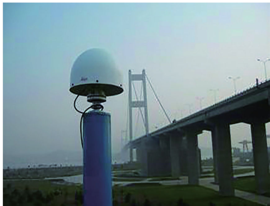
Fig. 4 Bridge deformation measurement by Beidou Satellite
