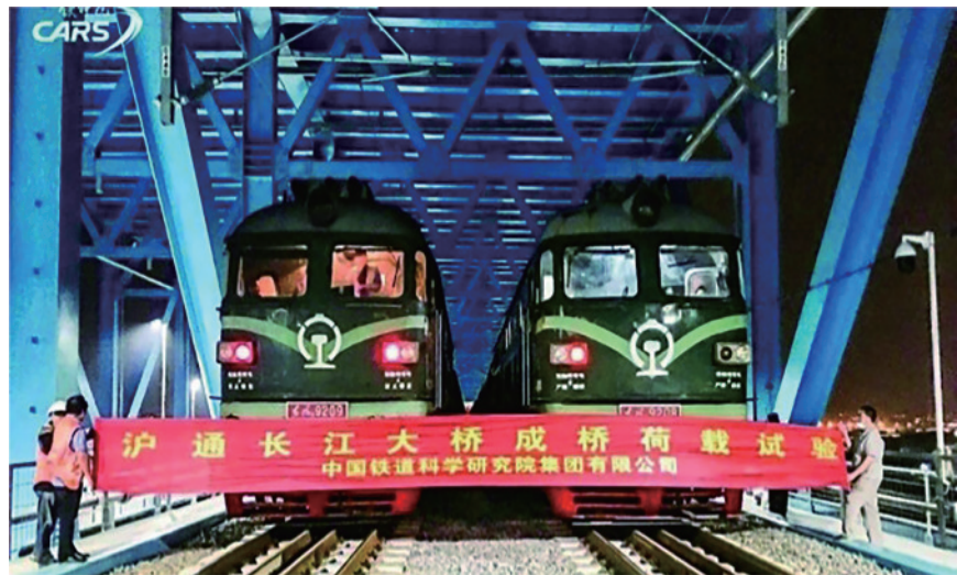
Fig. 9 Shanghai—Suzhou—Nantong Yangtze River Bridge completion test
