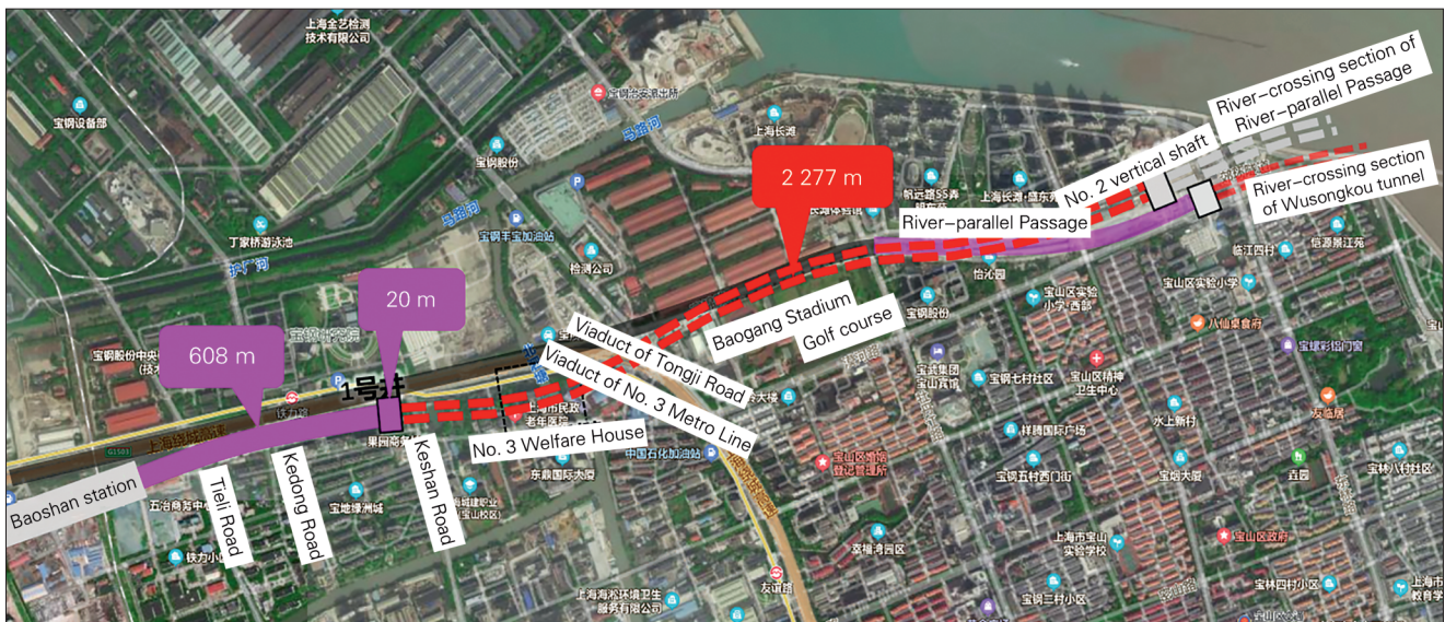
Figure 1 Plan of on-shore section of Wusongkou Tunnel
